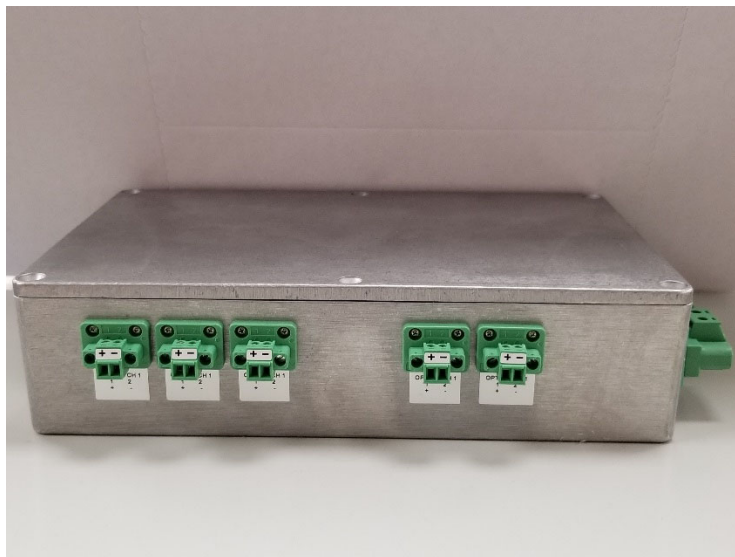
Figure 14: Output terminal for the Med-Vizion Distribution Box
