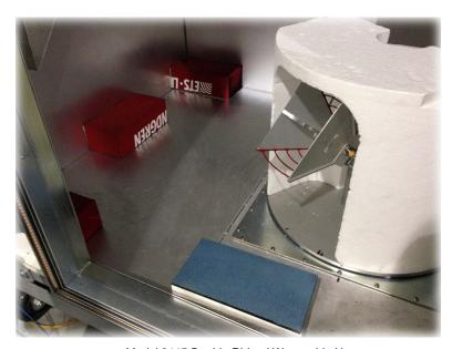
Model 3115 Double Ridged Waveguide Horn
