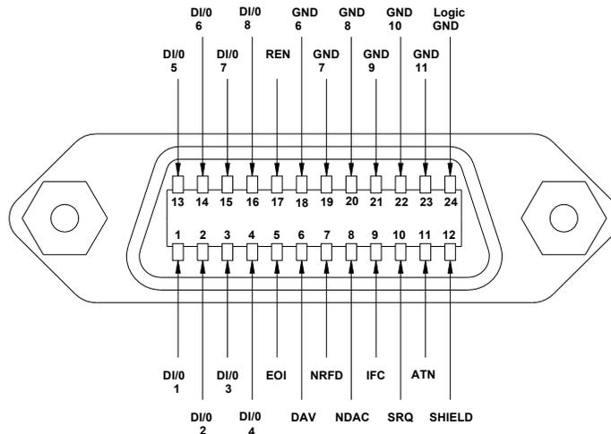
**Figure 7: Pin assignment of IEEE connector**
