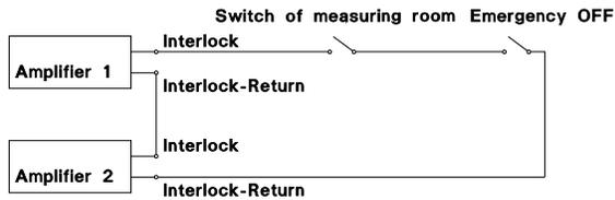
**Example of instruments with floating contacts which are referred to ground**
