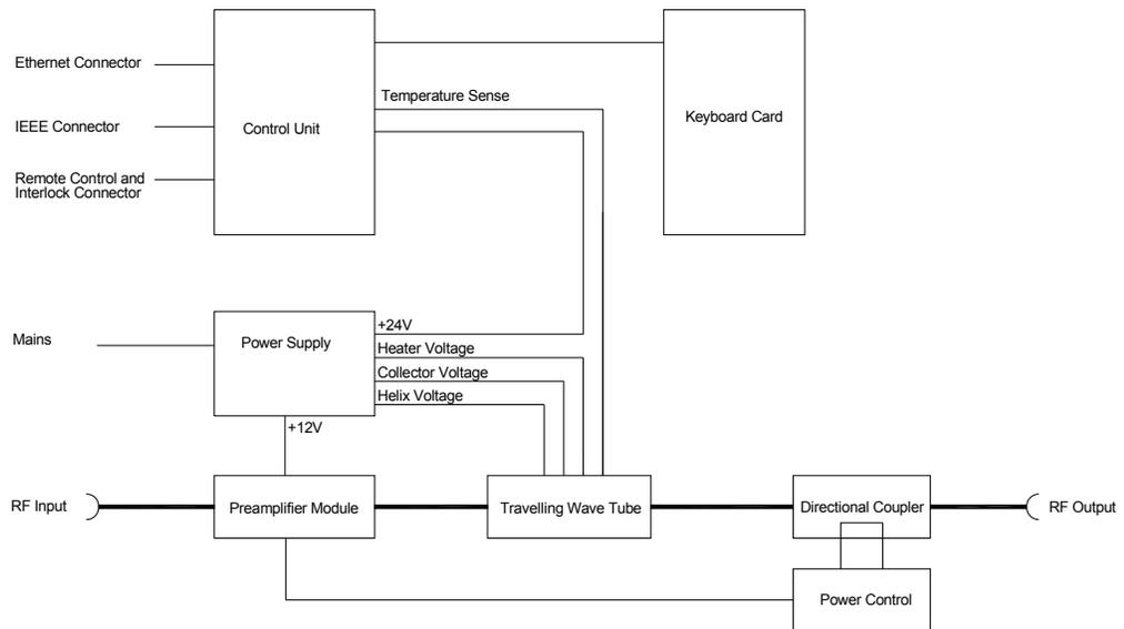
**Figure 1: Amplifier block diagram**
