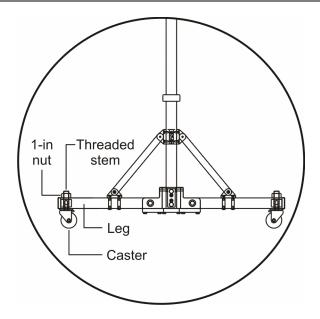
The casters include a threaded stem that can be rotated to raise or lower the extension leg. To adjust the height:
