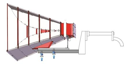
7. Attach the mounted assembly to the boom: Use the two 104136 knobs removed in step 1 to attach the antenna and mount adapter assembly to the boom. Tighten to secure.
