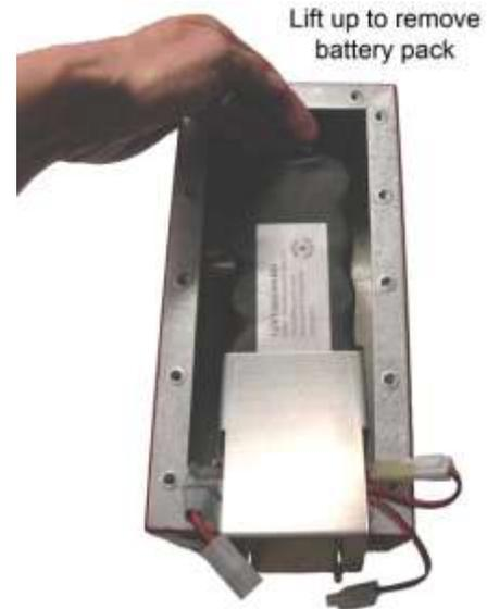
8. Place the new battery pack inside the enclosure.
