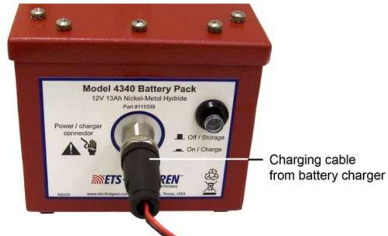
3. Plug the charging cable from the battery charger into the battery pack.
