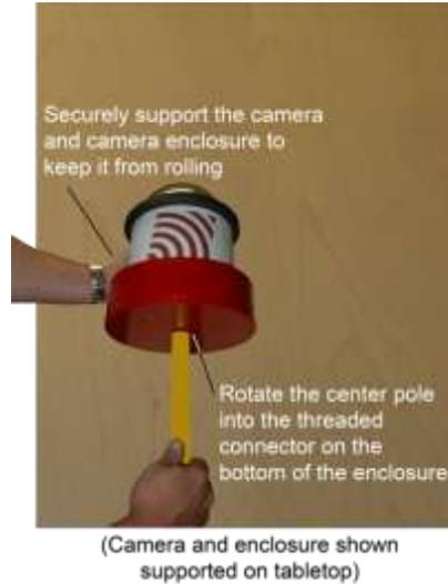
4. Supporting the camera and enclosure, carefully re-insert the 3/8-in thread center pole into the tripod. When the center pole is at the desired height, rotate the height adjuster knob to tighten.
