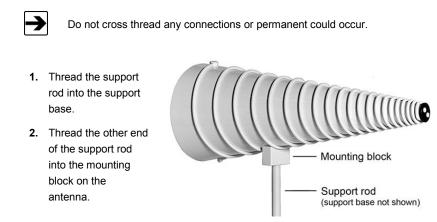
3. Attach the support base to the 4-TR, 7-TR, or mast.
