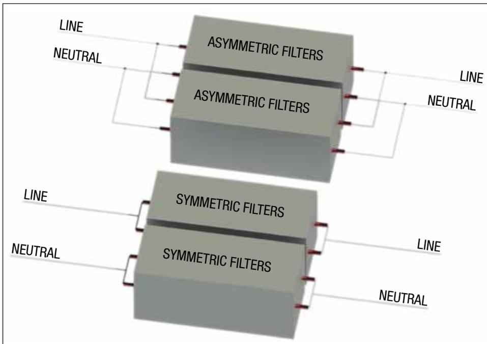
This diagram shows an example of the difference between paralleling asymmetric versus symmetric filters.
