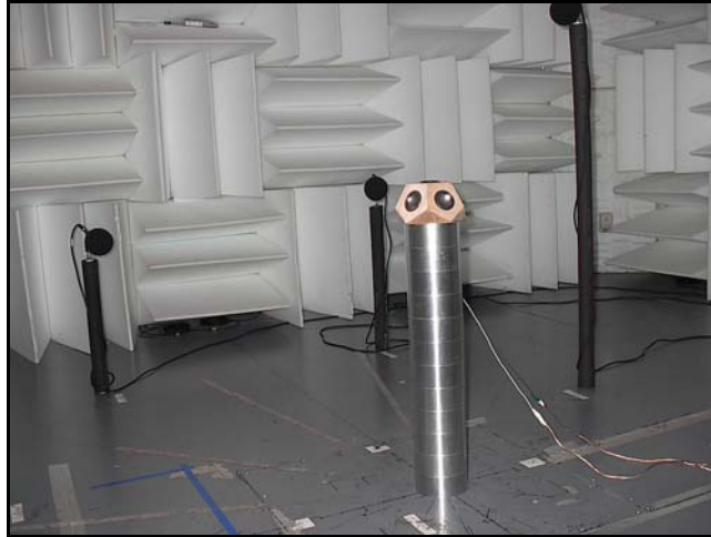
Figure 3: small loudspeaker cabinet raised underneath 1.4 meter radius ISO 3744 Table B.2 microphone array for “engineering method / grade 2” laboratory sound power determination.
