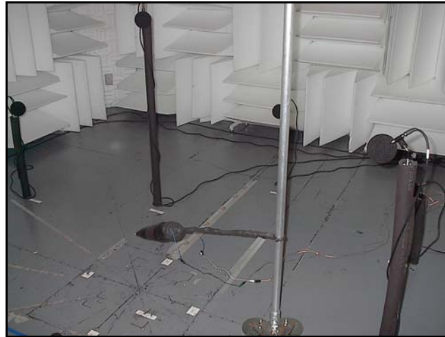
Figure 5: Tapered-cone loudspeaker suspended underneath 1.4 meter radius ISO 3744 Table B.2 microphone array for “engineering method / grade 2” laboratory sound power determination.
