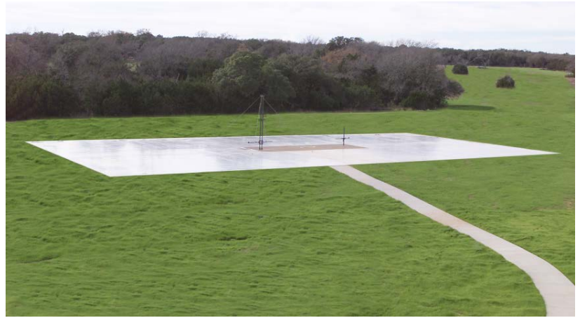
The outdoor metal ground plane at ETS-Lindgren's global headquarters in Cedar Park, Texas. At some 50 m x 80 m, the open area test site is part of ETS-Lindgren's A2LA accredited calibration lab, which has mutual recognition agreements with other worldwide laboratory accreditation systems, including ILAC. Laboratory equipment is NIST traceable and test processes are computer controlled for repeatability and data tracking.
