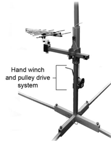
The mast is constructed of a high density fiberglass reinforced polymer with a high degree of immunity to structural deterioration from environmental elements. The base is an aluminum four-leg design for maximum support and portability. The design of the Model 1052 allows easy assembly and usage.
