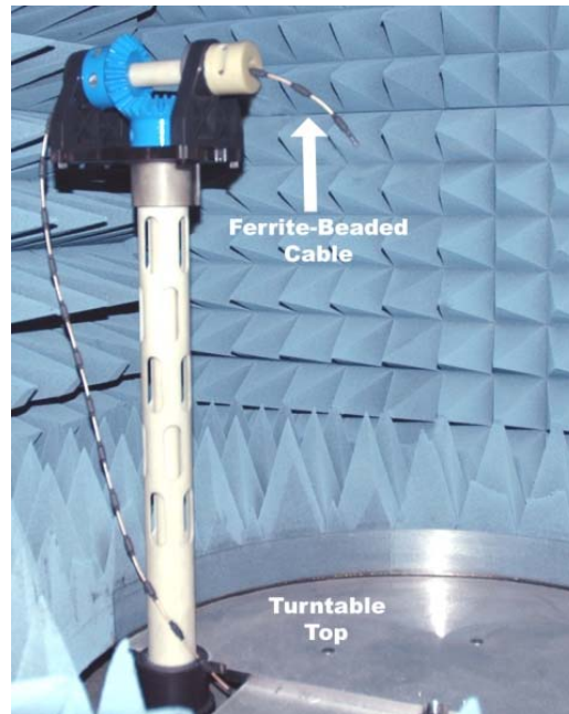
Figure 19: Ferrite Beaded Cable to the Top of the Turntable
