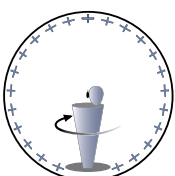
Multi-Antenna Distributed-Axis Scanning Method
