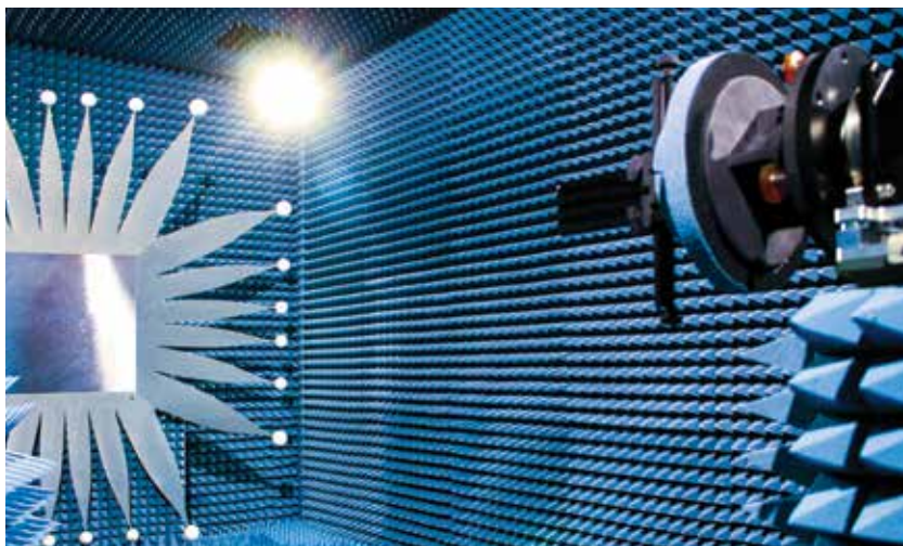
The AMS-5703 is ideal for 5G FR2 conformance and performance testing (EIRP, TRP, EIS, TIS), as well as radio interoperability testing.
