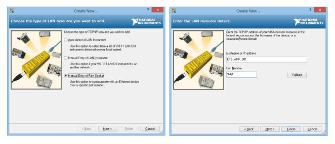
Launch VISA Interactive control. The amplifier will now be listed under 'TCP/IP Miscellaneous Resources'. Double click to open a connection.
