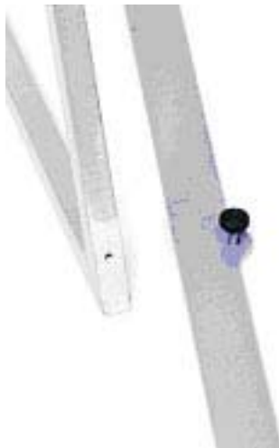
Figure 2: Bow-tie element receptacle hole and optional end plate with screw knob
