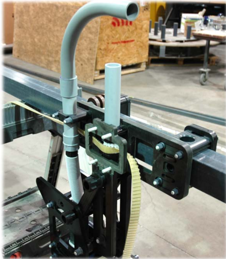
Thread the belt over the timing pulley.
