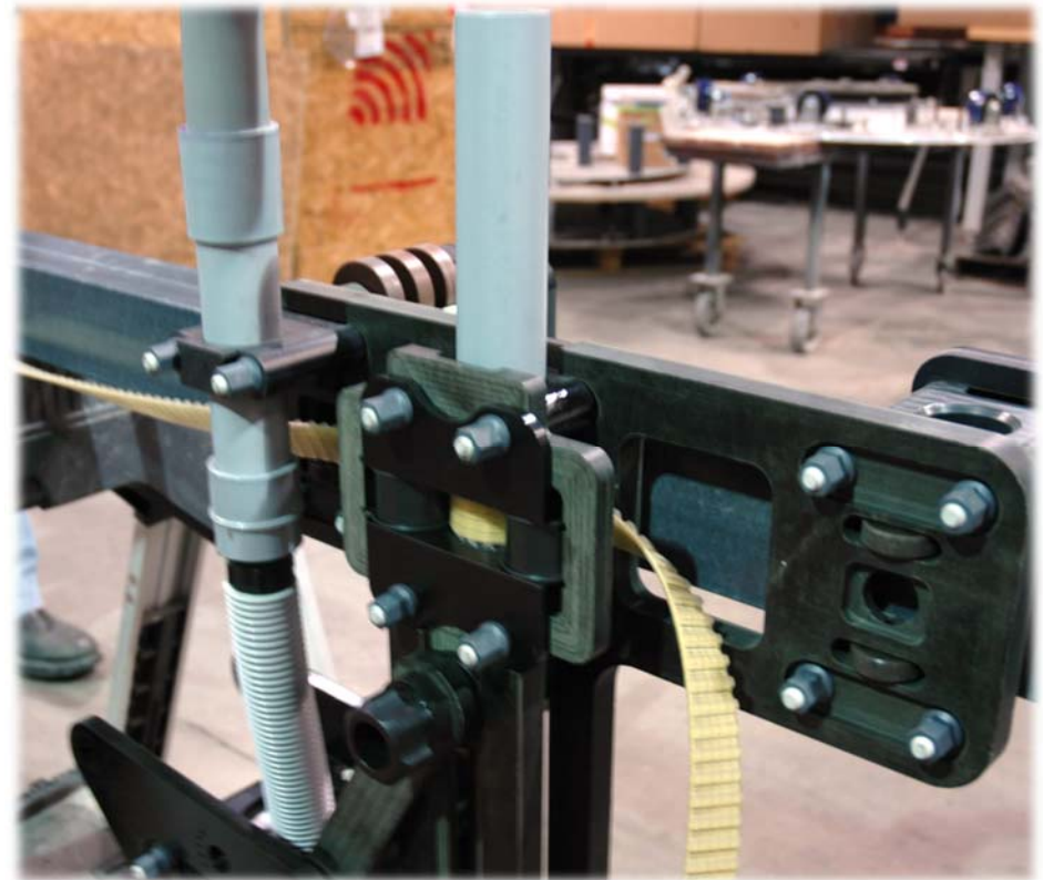
Replace the plate and four hex nuts to keep the belt in place while you move the mast into a vertical position; you will remove the plate and hex nuts again to adjust the timing in step 7 on page 37.
