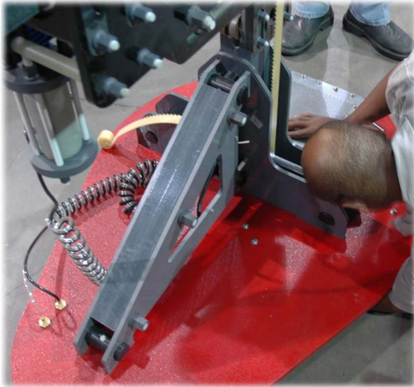
Reach under the base to access and remove the four cam followers with an Allen wrench.
