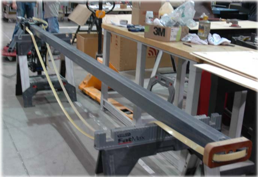
Route the belt to the top of the mast, over the pulleys, and down the other side of the mast.
