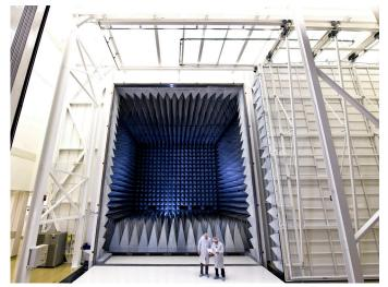
ETS-Lindgren installed a large RF shielded anechoic chamber for Passive Intermodulation (PIM) emissions testing of satellites at the Lockheed Martin Company (LMCO) production facility in Sunnyvale, California. Certifying that a LMCO satellite is not producing PIM emissions expedites development schedules, allowing LMCO to better meet commitments to its customers.
