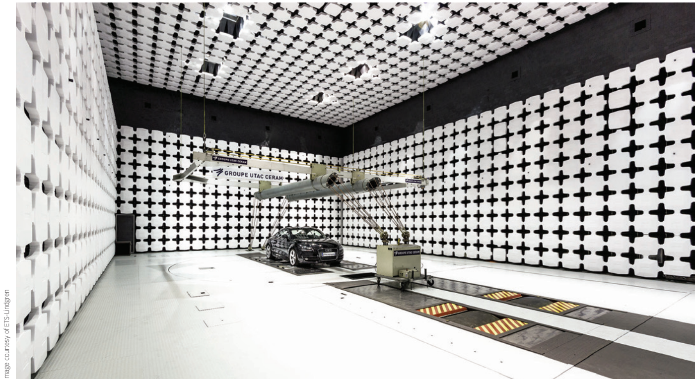
Photo 1: Automotive test chamber using polystyrene absorber
